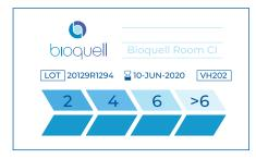
The Bioquell Room CI without any exposure to hydrogen peroxide vapour
