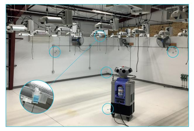
*Figure 1.* Bioquell hydrogen peroxide vapor generator located within one of the grow rooms. Biological indicators are positioned at various locations around the enclosure (marked, but not all shown).
